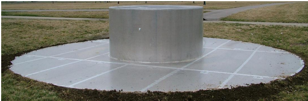
Figure 6. Digital picture reference of the calibrated tophat reflector used in the calibration array of the spotlighted scene center.
