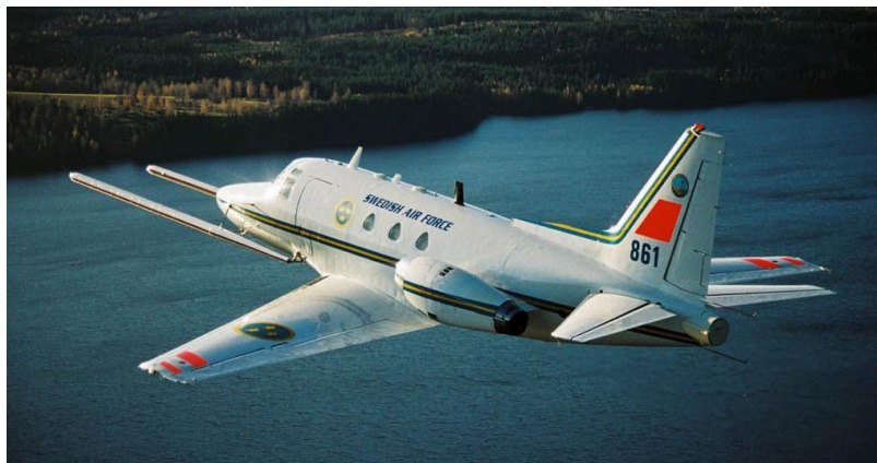
Figure 1. The CARABAS-II VHF SAR in operation with the antennas deployed in the front of a Sabreliner aircraft (© Photo: Pia Ericson, FMV).
